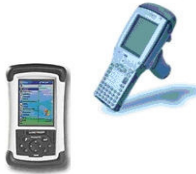
Portable devices for reading RFID-tags in offline and online mode for industrial service
